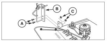
Figure 12. Anchor Bracket Installation
